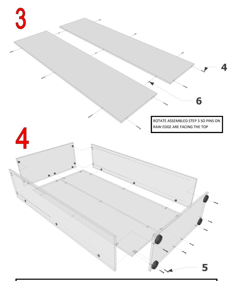
ALIGN SIDES WITH BACK, PUSH IN PLACE AND TIGHTEN TIGHTENING SCREW UNTIL SECURE
